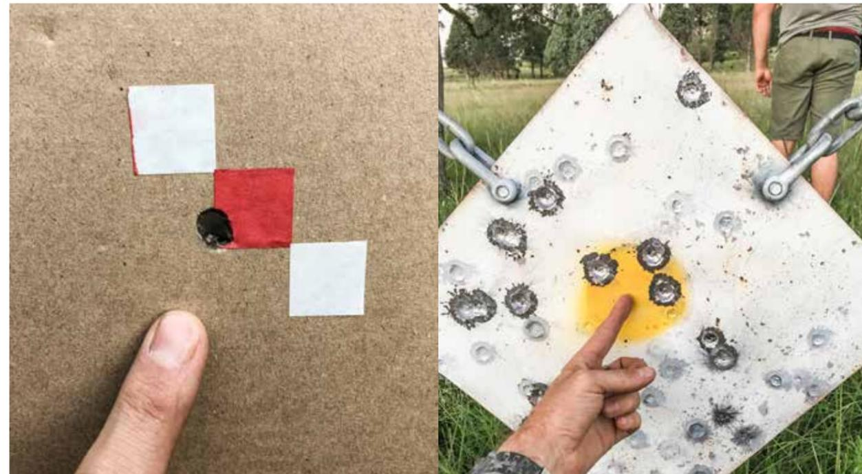
▲ A 100m group like this doesn't necessarily equate to a 900m group like the image on the right. The 100m group could be achieved with an ES of 150fps, which however would result in a 0.9mils / 3.09MOA vertical dispersion @900m in a 338LM. A chronograph is thus essential to monitor velocity consistency before selecting your load.
